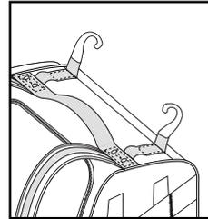
2 plastic hooks located on backpack straps are used to hang bag onto fence.
